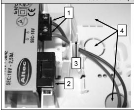
To connect to the electric power 230VAC, use a cable with 2 voltage connectors of 1.5 mm<sup>2</sup>
